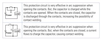
Generally, switching a DC inductive load is more difficult than switching a DC resistive load. Using an appropriate arc suppressor, however, will improve the switching characteristics of a DC inductive load.
